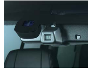
Automatic high beam (camera shown) 📷 21
