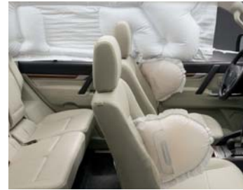
Front seat side and curtain SRS airbags 📷 04
