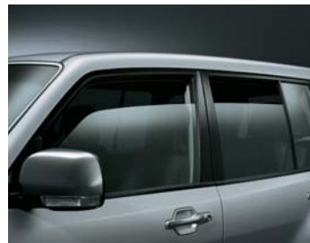
Power windows with time-delay and driver's auto-down function 📷 13
